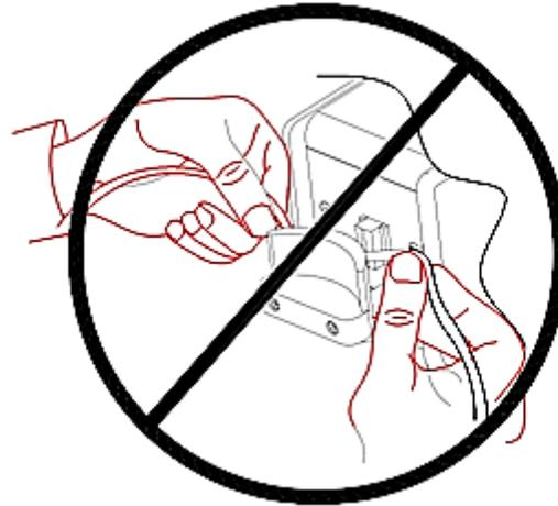
Figure 3-2, Incorrect Technique for Holding the Tubing
