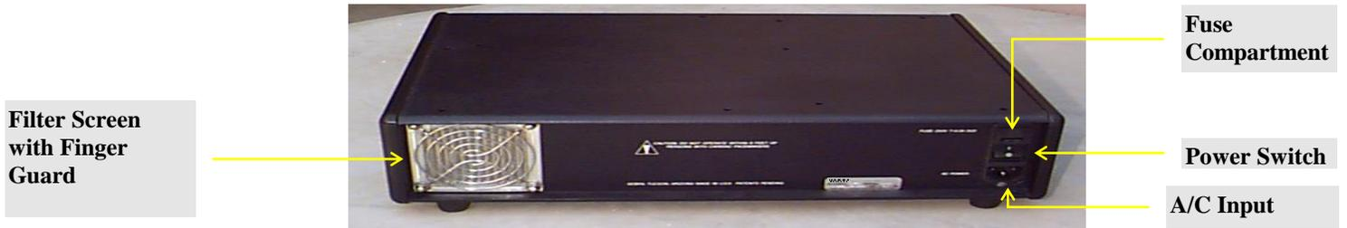
Figure 1.2 Model 3120 RF Generator Rear View
