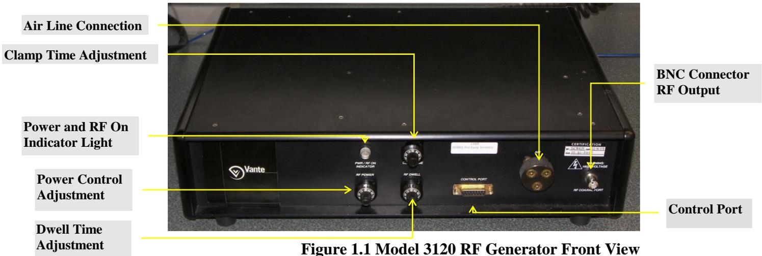
Figure 1.1 Model 3120 RF Generator Front View
